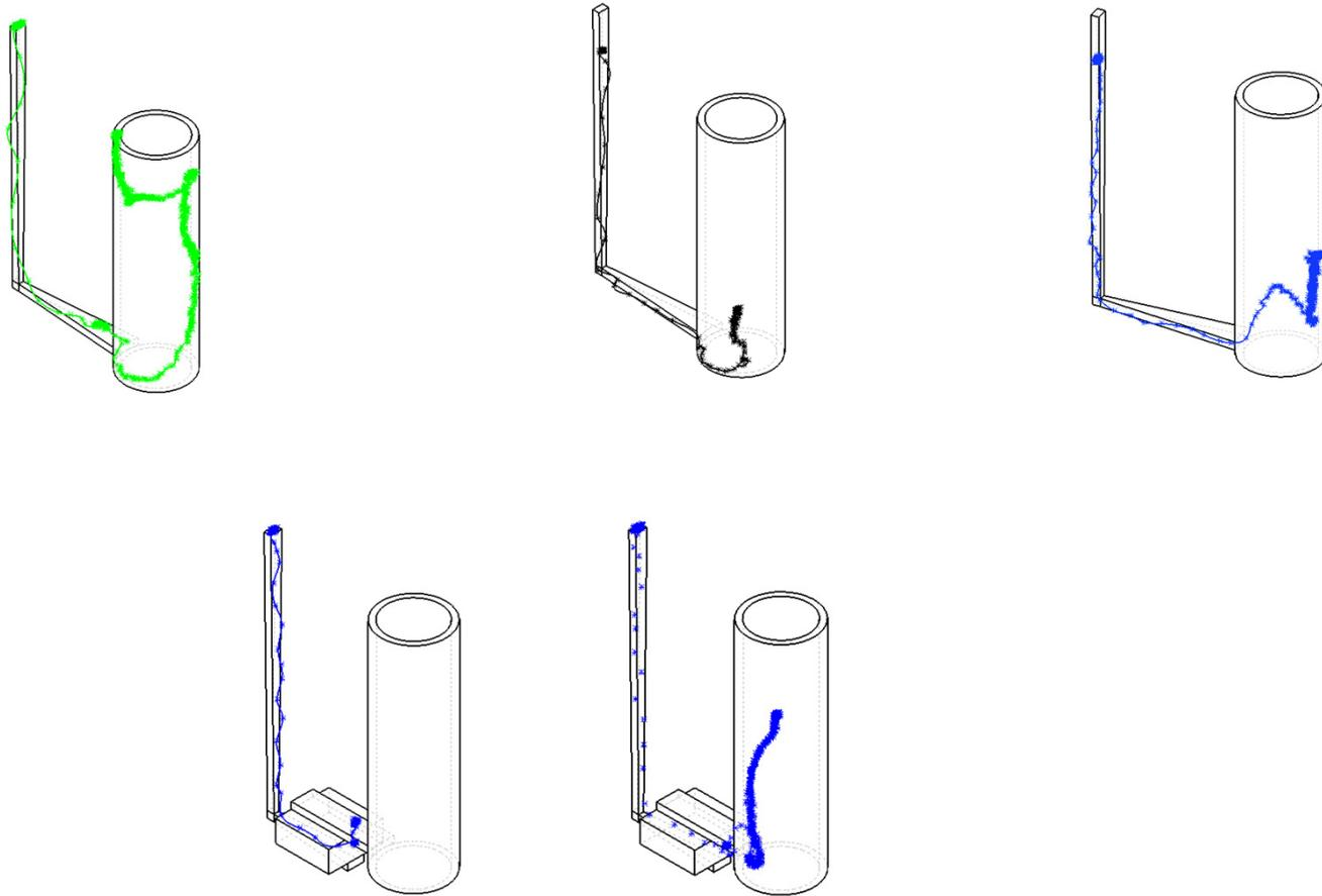
Examples of the use of PEPT to study filtration of liquid metal using ceramic foam filters. In (a) the alumina particle has become trapped in a 30 ppi filter. In (b) the alumina particle has passed through a 20 ppi filter.
