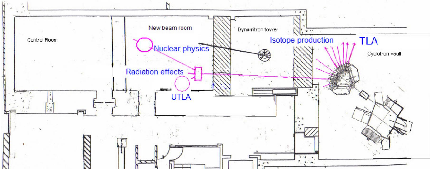
More recently, we were asked to provide high dose-rate damage studies (LHC ATLAS group and metallurgy) so extended a second beam-line into a specially shielded area.
