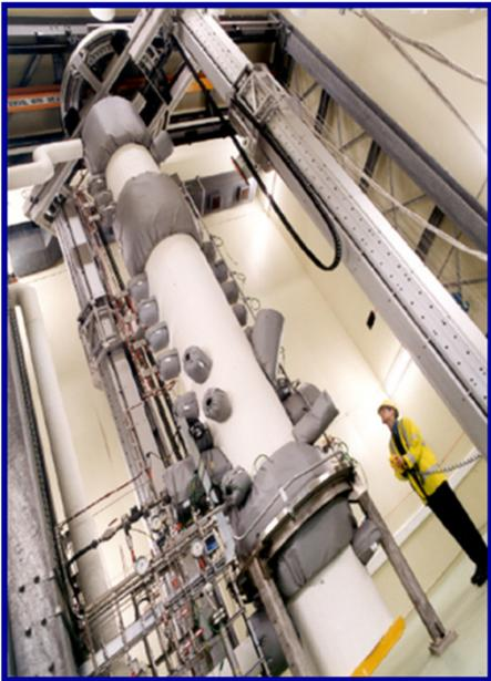
750mm diameter fluidised bed, with central dividing baffle + different air supplies each side of baffle
