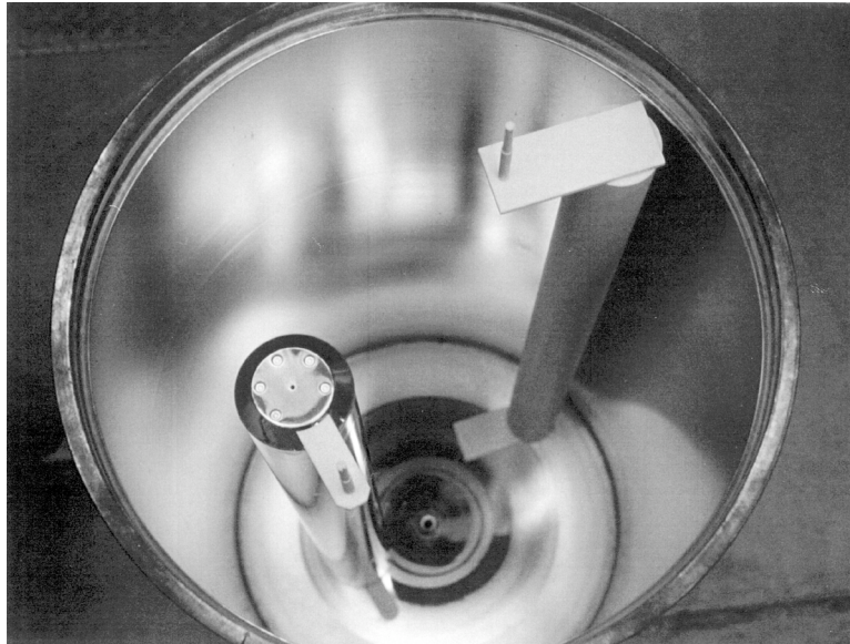
Figure 3.2. The resonant cavity viewed from above with the top flange removed. The diameter is 50cm and the depth is 1m.
