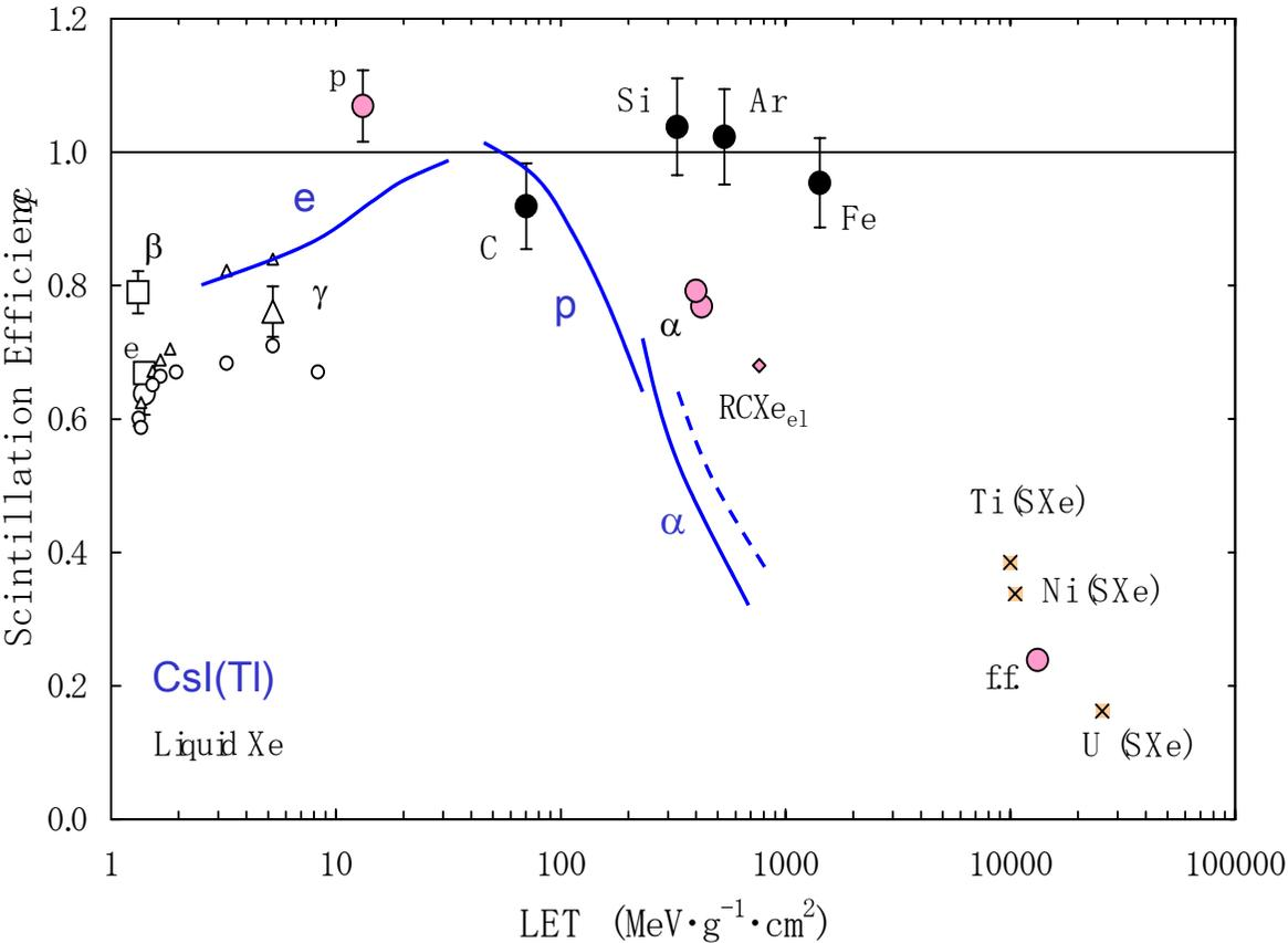
Fig. 2 Scintillation efficiency for various ions as a function of the electronic LET for liquid Xe and CsI(Tl).
