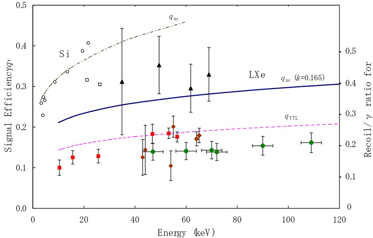
Fig. 4 Scintillation efficiency for recoil ions in LXe as a function of recoil ion energy. The nuclear ( $q_{nc}$ : Lindhard) and the total ( $q_{TTL}=q_{nc} \times q_{el}$ ) quenching factors are shown. The results for Si are also shown for comparison.  $q_{el}$ : exciton-exciton collision model
