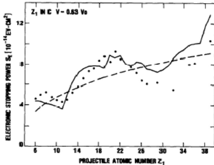
Fig. 1. Electronic stopping power as a function of projectile ion at the velocity  $v = 0.63 v_0$  in a carbon target: — present values; - - - Lindhard-Scharff values; ··· data from Aarhus<sup>10</sup>
