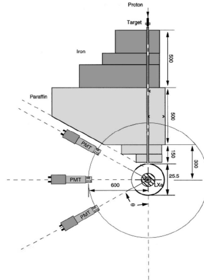
Fig. 3. Top view of the experimental setup at the LNL neutron beam line.
