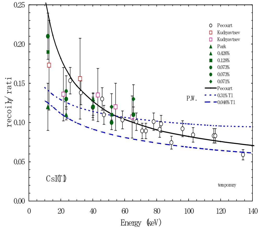
Fig. 3 The recoil ion to  $\gamma$  ratio in CsI(T) as a function of recoil ion energy. The broken lines are present estimates. The solid line is fitting to the Birks-Lindhard model by Pecourt.
