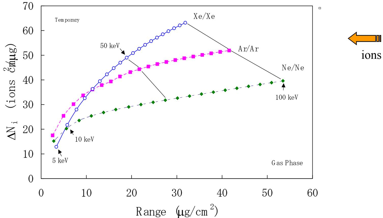
Fig. The electronic LET,  $d\eta/dR_T$  for recoil ions in rare gases. The ions enter from the right hand side. Points are plotted at every 5 keV. Used for the electronic quenching calc in condensed media.
