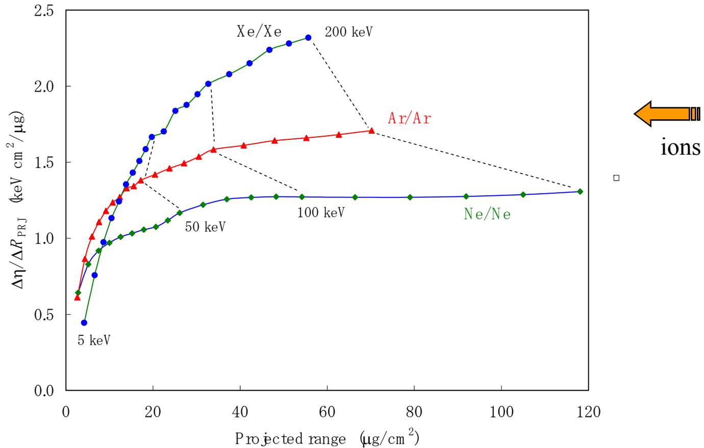
Bragg-like curves,  $d\eta/dR_{PRJ}$  for recoil ions in rare gases.
