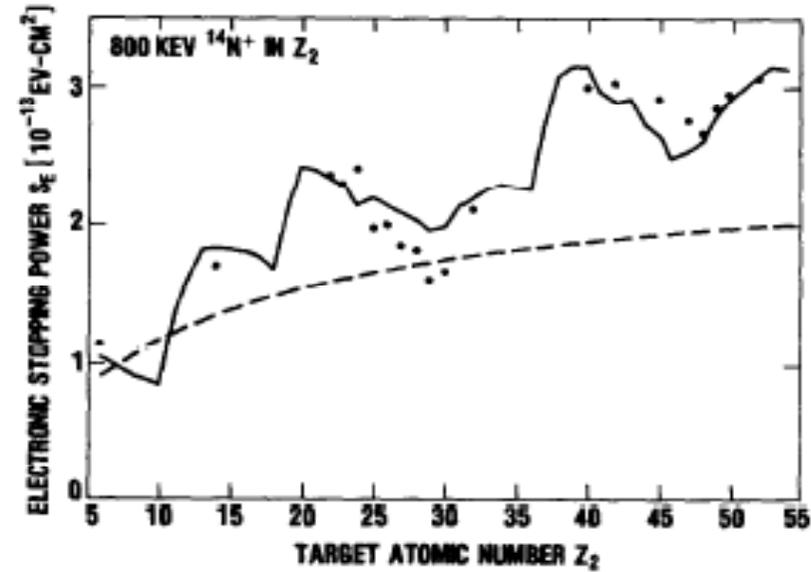
Fig. 2. Electronic stopping power as a function of target atom for incident 800-keV nitrogen ions ( $v = 1.51 v_0$ ): — present values; - - - Lindhard-Scharff values; ··· data from NAVSWC<sup>6,7</sup>
