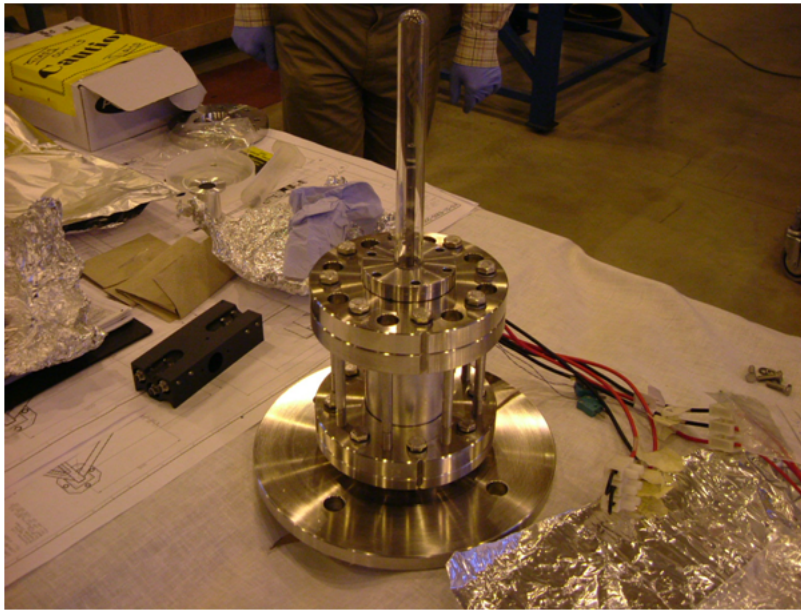
Figure 6.9: The glass tube on top of the stator can be seen in this photograph with a prototype optics block loaded with collimators on the left.
