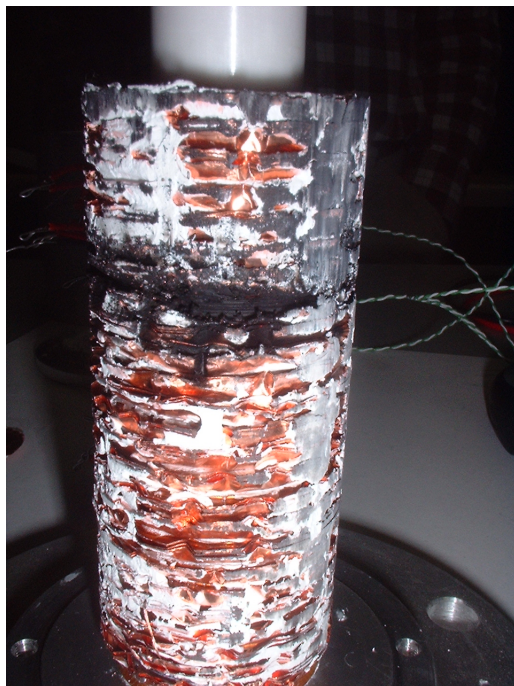
Figure 10.1: A photograph of the coil stack clearly showing the location of the coil failure.
