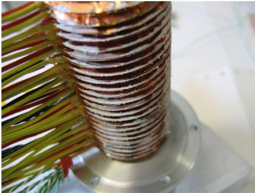
Figure 5.5: All 24 coils assembled on a former. The copper shims can be clearly seen protruding from the coil stack where they will later make contact with the cooling jacket.
