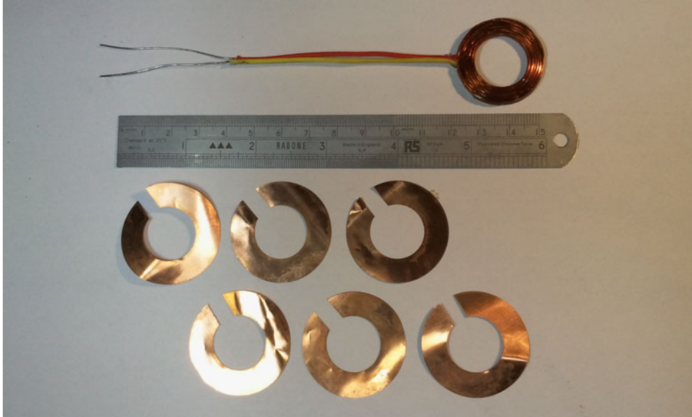
Figure 3. A complete stator coil and some copper heat-sinking shims.
