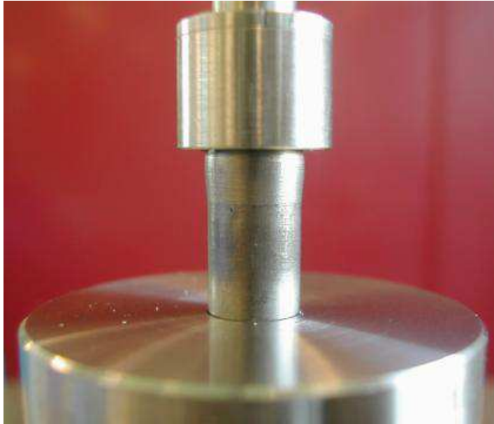
Figure 14: A bulge can be seen in the shaft under the stop. This occurred during impact testing.
