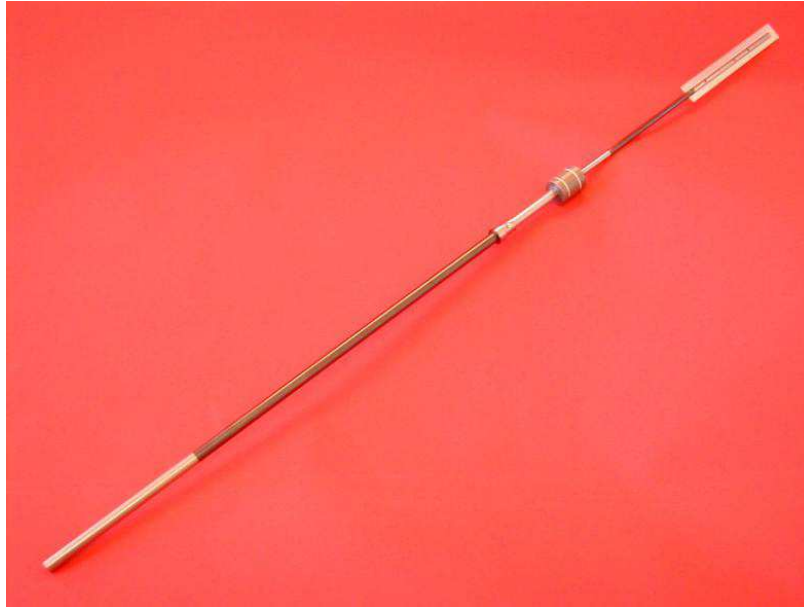
Figure 16: DLC coated shaft, dark grey/black coating extending over and beyond the bearing regions of shaft.
