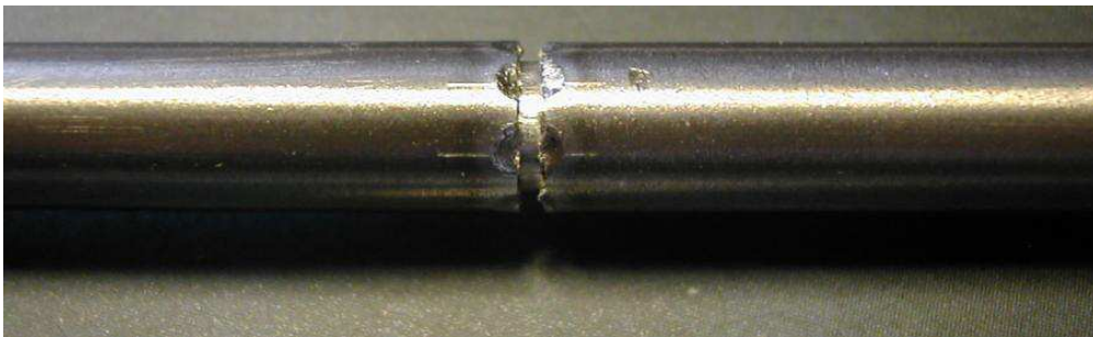
Figure 13: Failed weld and displacement of shaft halves after tensile testing
