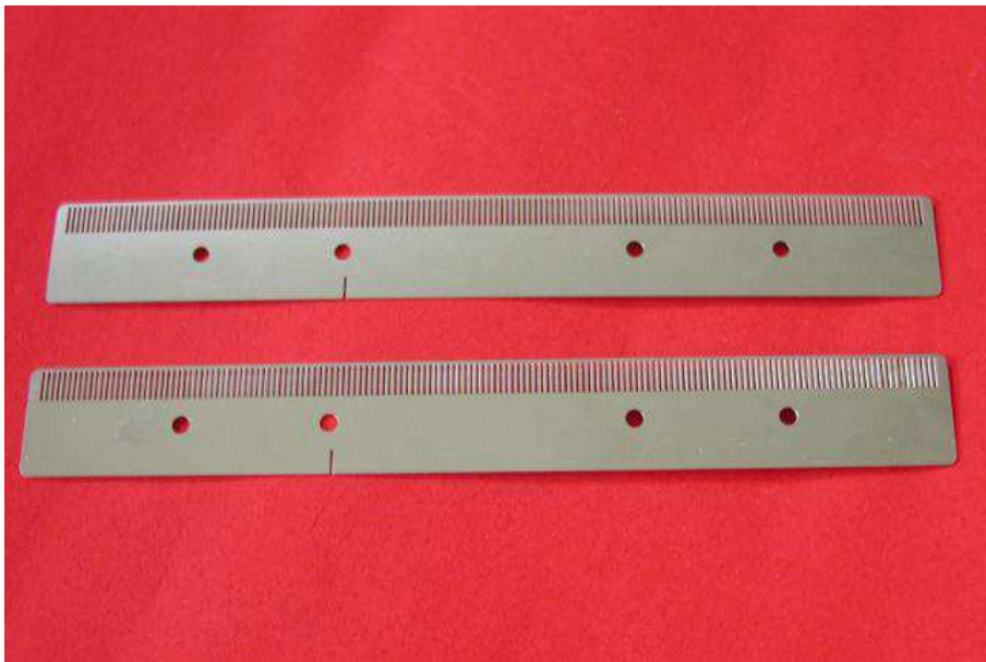
Figure 26: Two optical vanes. One side has 157 apertures to provide a quadrature signal. The other has a single slot to give a fixed reference point.
