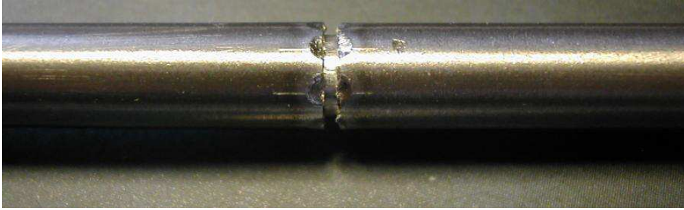
Figure 12: Failed weld and displacement of shaft halves after tensile testing
