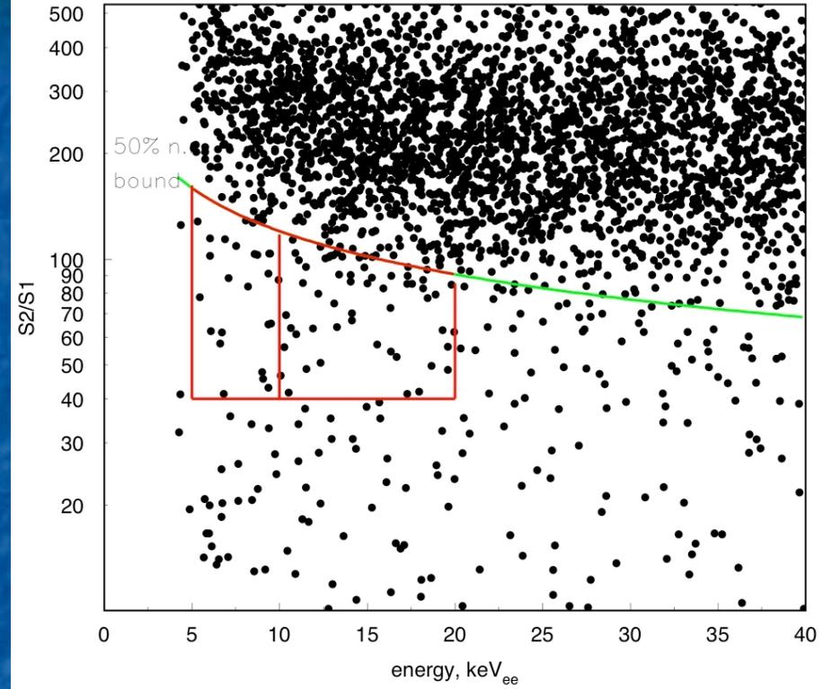
Red box - 50% nuclear recoil acceptance box defined using calibrations and unblind 10% of data;  $S2/S1 > 40$ ,  $S1$  (energy) = 5 - 20  $\text{keV}_{ee}$ .
