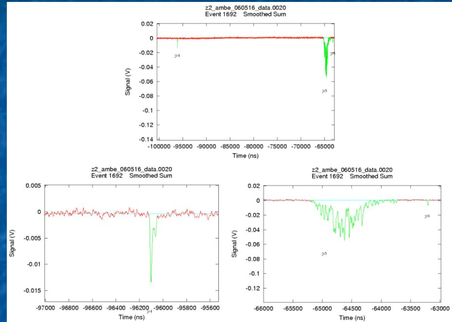
Electron recoil pulse from the dark matter run
