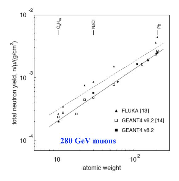
A-dependence of neutron production rate -GEANT4 v6.2: Araujo et al. NIMA <u>545</u> (2005), 398; GEANT4 v8.2: Lindote et al., in preparation; FLUKA: Kudryavtsev et al. FLUKA gives twice as many neutrons as
