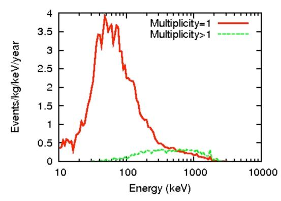
Energy spectrum of single electron recoils from U in stainless steel vessel behind inner shielding: lead and polyethylene - more events at low energies due to the presence of polyethylene close to the crystals.
