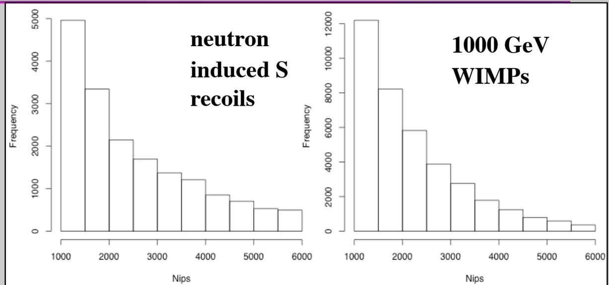
**(left) Monte Carlo spectrum >1000 NIPs of S recoil zenith angles (z axis) from z-directed  $^{252}\text{Cf}$  neutrons; and (right) equivalent for 1000 GeV WIMP wind. The WIMP induced recoils are peaked slightly higher (using GEANT)**
