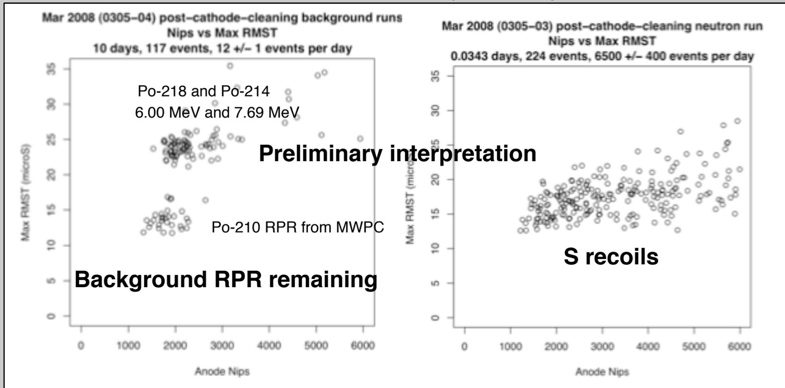
Preliminary interpretation: (i) remaining short-life cathode RPRs can be cut and reduced by flushing, (ii) remaining MWPC RPRs (~1/day)
