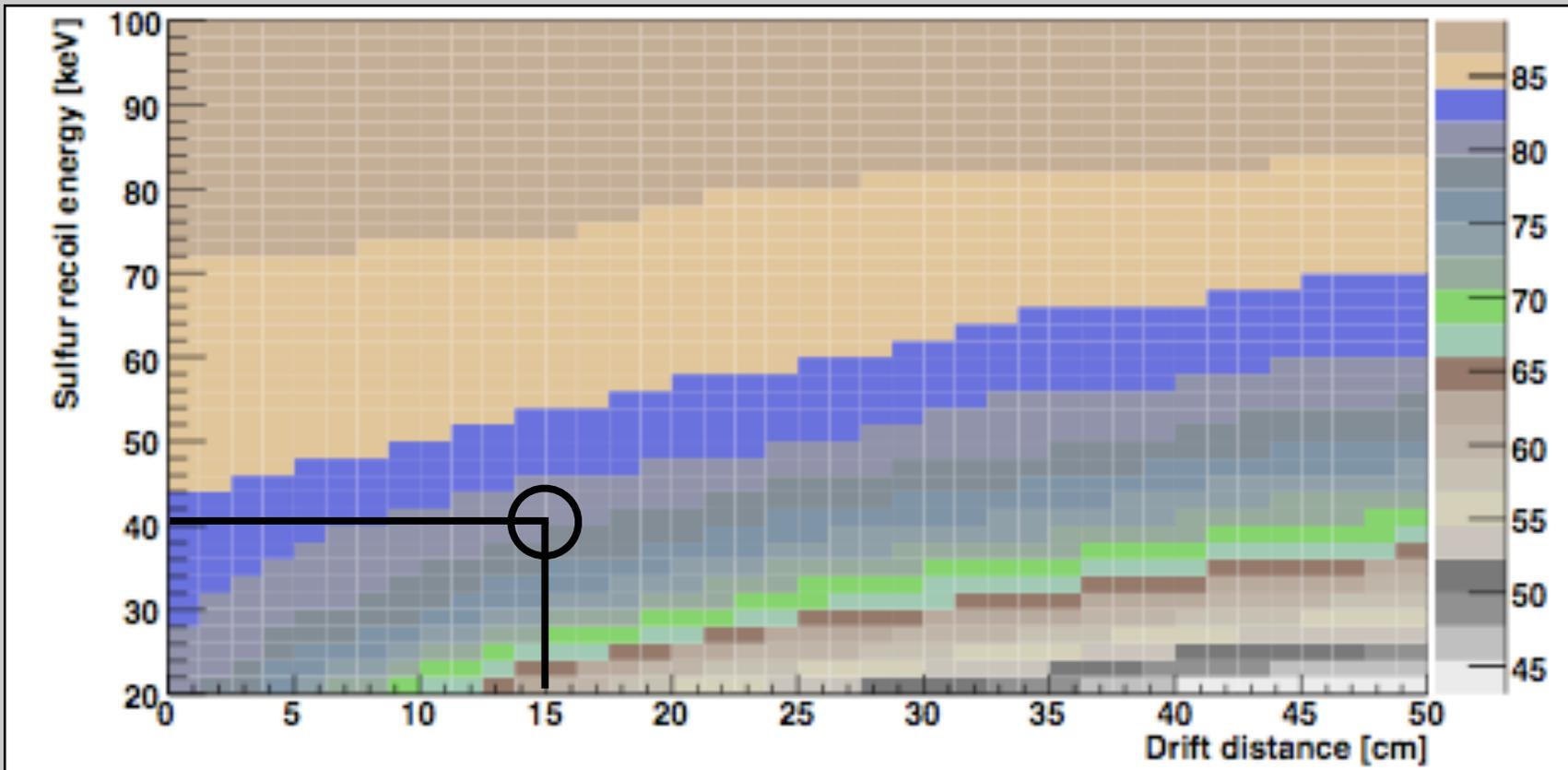
e.g. for 15 cm drift distance 75% of 40 keV S recoils reconstructed within  $30^\circ$  of initial direction
