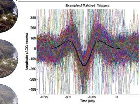
Left: An example of triggers pattern matched to the bold signal shape (derivative of bipolar) by the matched filter. Right: An example of recurring signal types identified (from top): 50kHz oscillating low freq. oscillating impulsive 10kHz sinusoidal ringer 'bipolar' [y-axis: P(Pa); x-axis: sample №]
