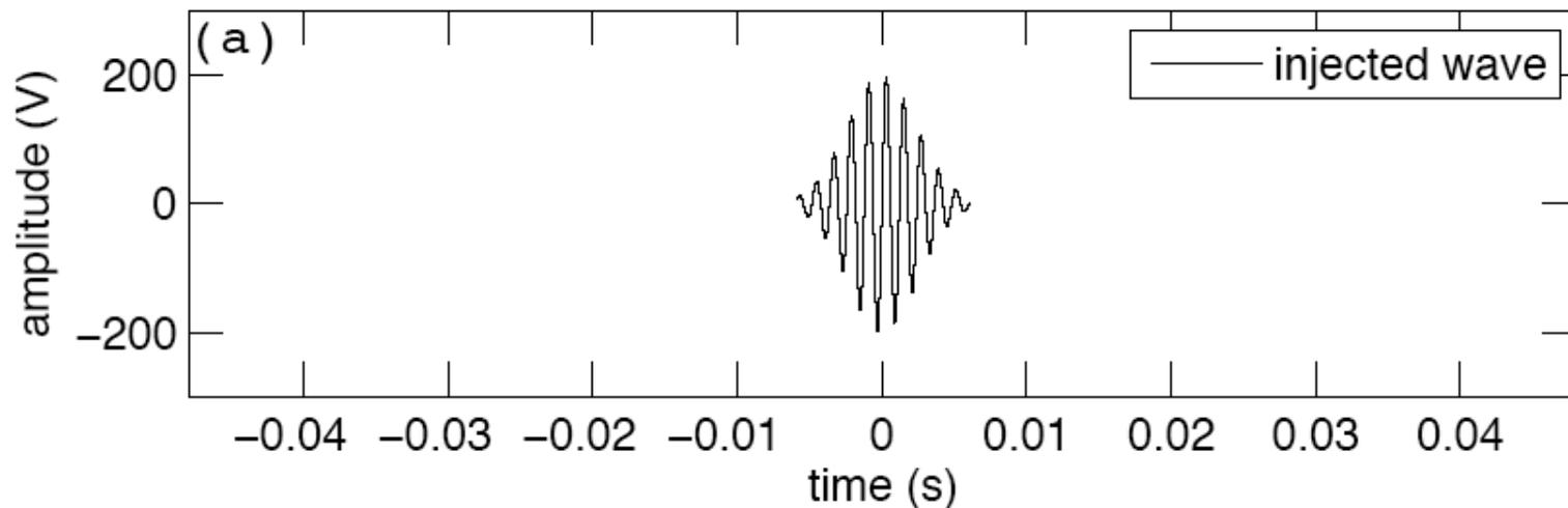
How might you look for a signal like this? Common sense suggests setting a threshold in amplitude, then looking for coincidence between signals at multiple instruments.
