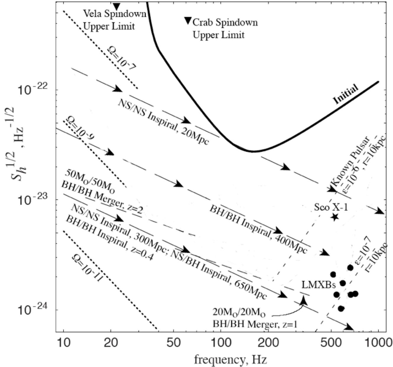
Where source has strain amplitude equal to or greater than IFO noise on this plot, source is detectable on background noise with a 1% false acceptance rate.
