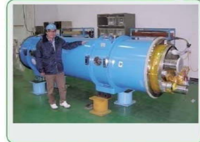
Combined dipole-quadrupole SC magnet
