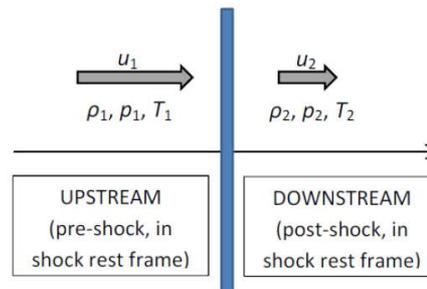
$$\begin{aligned}\rho_1 u_1 &= \rho_2 u_2 \\ \rho_1 u_1^2 + p_1 &= \rho_2 u_2^2 + p_2 \\ \frac{p_1 \gamma_g}{\rho_1 (\gamma_g - 1)} + \frac{1}{2} u_1^2 &= \frac{p_2 \gamma_g}{\rho_2 (\gamma_g - 1)} + \frac{1}{2} u_2^2\end{aligned}$$
